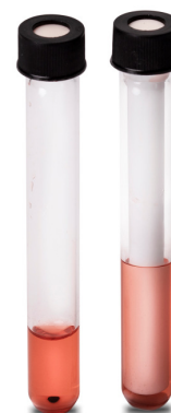
Solstice reactor tubes with and without Thin-film insert (1.5ml solution volume)
