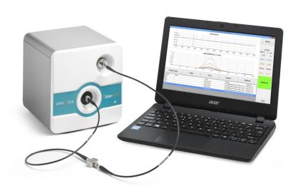
Typically used to monitor steady state conditions and control product collection in flow-through applications, the high pressure flow cell, which uses PFA or FEP tubing and connects to the source and detector module using fibre optic waveguides, may be inserted virtually anywhere in the flow path.
